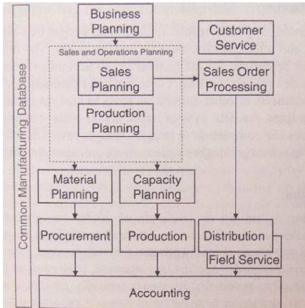
Fig. - Architecture of an ERP System
